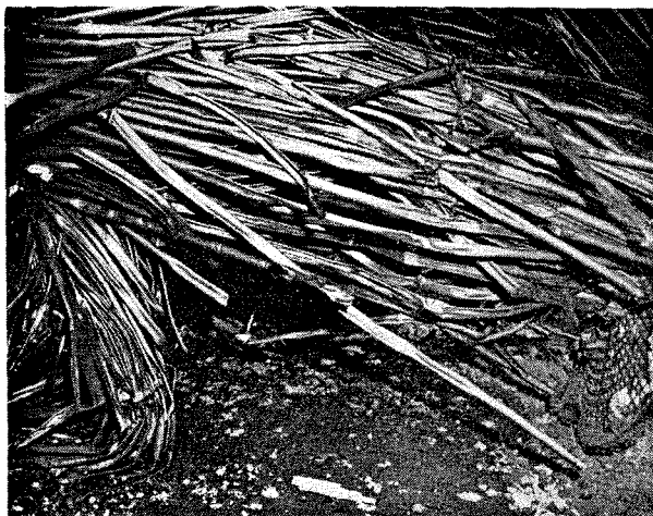
Figure 3. Close-up of tubes in vaporizer and bottom tube sheet at right. The line of detonation can be seen to be approx. 6-8 in. above the tube sheet.
